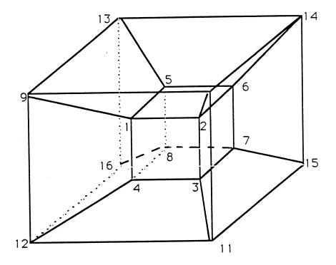
Figure 3. The hypercube connectivity graph
