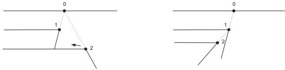
Figure 2: A pivot event. As s_2 moves left, s_0 , s_1 and s_2 become collinear.
