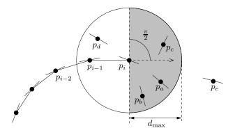
Figure 3: Extending the path  $P = (\dots, p_{i-2}, p_{i-1}, p_i)$  at the end point  $p_i$ . Only points in the gray area can be linked. The maximum distance allowed to link points is  $d_{\text{max}}$ .
