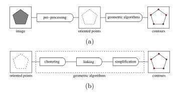
Figure 2: Overview of our method. (a) Two stages. (b) Geometric algorithms for the second stage.
