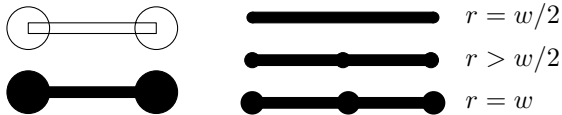
Figure 1: Left, an edge is drawn as a rectangle that connects two centers of vertices in the natural way. Right, a graph with three vertices and two edges, and different ratios of r and w .
