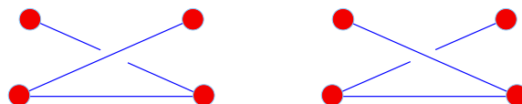
Figure 1: Two conformations which are geometrically close but kinetically far away. Red dots and blue lines denote atoms and bonds respectively.
