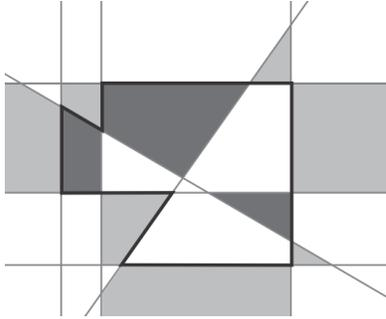
Figure 2: Example of internal shadow and external light faces of a polygon.
