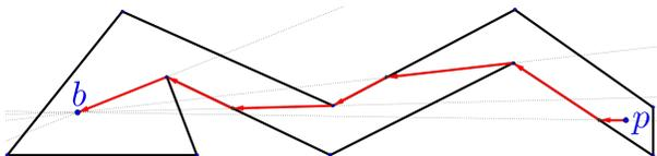
Figure 1: The movement of a point alternates between moving straight towards the beacon and sliding on the boundary.
