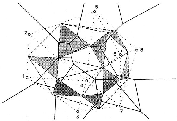
$Del_1(S)$  (dotted lines),  $Del_2(S)$  (dashed lines) and  $Vor_2(S)$  (solid lines); 3,4,6,8 are cocircular and neutral regions of  $Del_2(S)$  are in grey.
