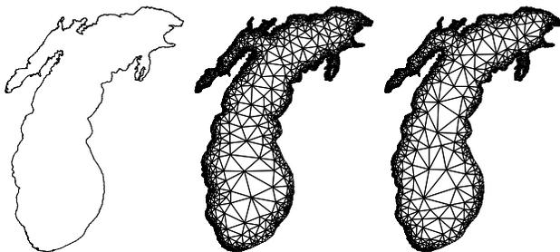
Figure 1: Using the boundary of Lake Michigan as input (left, 1537 vertices) and a minimum angle threshold of  $25^\circ$ , the results of Ruppert’s algorithm (center, 3707 vertices) and Chew’s second Delaunay refinement algorithm with off-centers (right, 2960 vertices) are shown.
