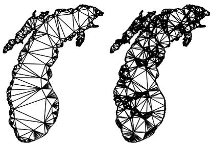
Figure 6: Meshes produced using  $\alpha^* = 5^\circ$  with  $\Upsilon = 6^\circ$  (left, 1660 vertices) and  $\Upsilon = 59.5^\circ$  (right, 6072 vertices).
