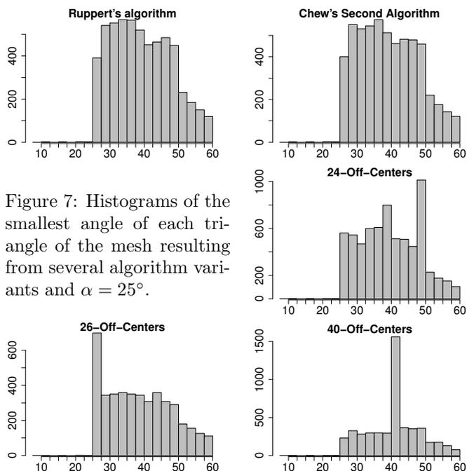
Figure 7: Histograms of the smallest angle of each triangle of the mesh resulting from several algorithm variants and  $\alpha = 25^\circ$ .
