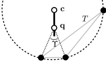
Figure 4: For a poor quality triangle  $T$ , the set of admissible  $\Upsilon$ -off-centers is shown with the triangle circumcenter  $\mathbf{c}$  and a typical  $\Upsilon$ -off-center  $\mathbf{q}$ .
