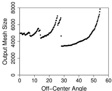
Figure 8: The number of vertices in the resulting mesh using  $\Upsilon$ -off-centers for various values of  $\Upsilon$  and  $\alpha = 25^\circ$ .
