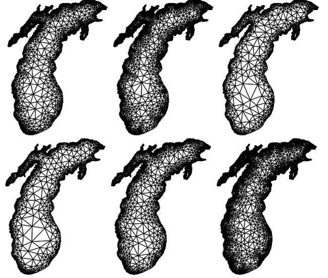
Figure 5: Meshes produced using  $\Upsilon$ -off-centers,  $\alpha^* = 28^\circ$ . (top left)  $\Upsilon = 0$  (i.e., circumcenter insertion) gives 4975 vertices. (top center)  $\Upsilon = 27 \Rightarrow 6475$  vertices. (top right)  $\Upsilon = 29 \Rightarrow 3432$  vertices. (bottom left)  $\Upsilon = 40 \Rightarrow 3955$  vertices. (bottom center)  $\Upsilon = 50 \Rightarrow 5346$  vertices. (bottom right)  $\Upsilon = 55 \Rightarrow 8617$  vertices.
