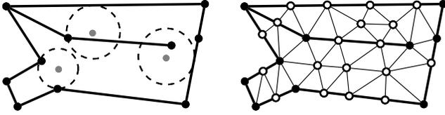
Figure 2: A PSLG (left) with local feature size indicated at several points (gray) and a refinement (right) of the PSLG that gives a quality, conforming triangulation.
